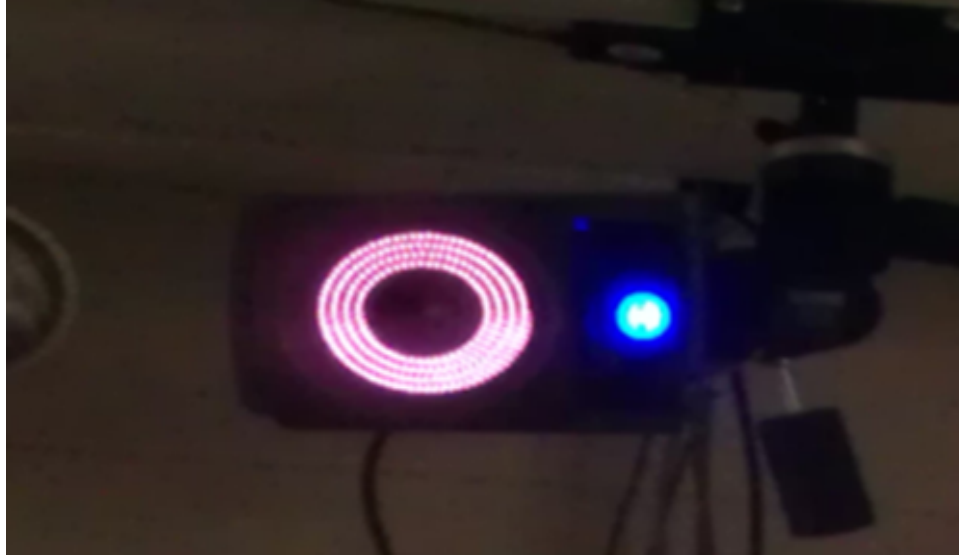
Figure 13. VICON Motion Capture Camera. T-series VICON motion capture camera, with millimeter resolution, was used to capture the spatial coordinates of the subject of interest (SOI). The markers situated on the SOI reflect the IR radiation emitted by the LEDs on the camera.
