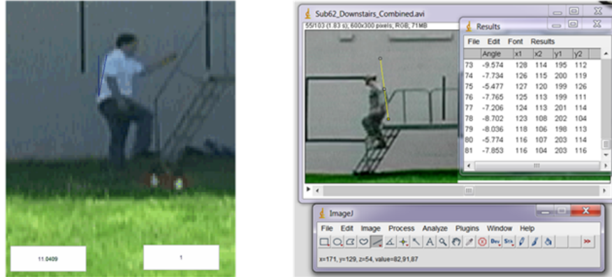
Figure 3. MATLAB GUI and ImageJ. The MATLAB GUI (left) and the ImageJ (right) were both used to analyze the back angle and these interfaces calculated these angles for each trial frame by frame. Two vectors were drawn manually by the user and the angles between them were measured and recorded [11].
